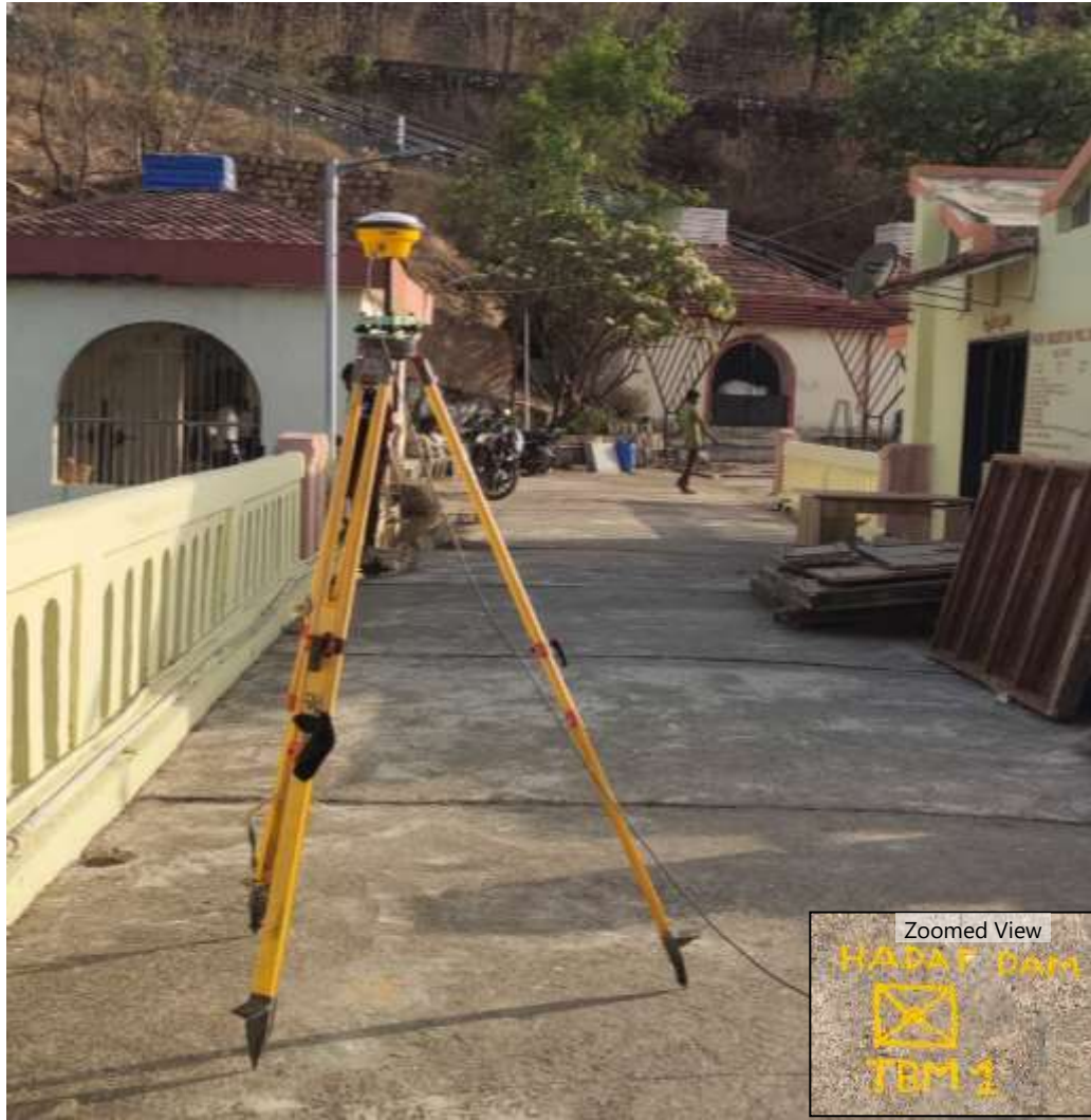
Figure 3.1: Hadaf Dam Temporary Benchmark (Hadaf Dam TBM 1)
